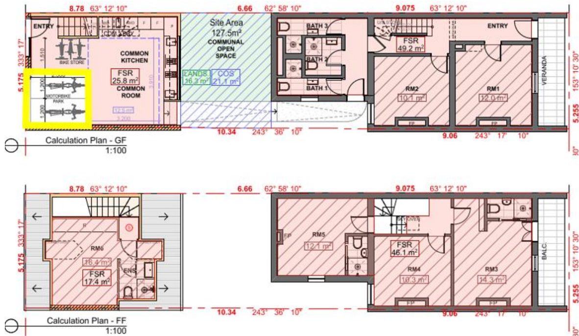
Figure 26: Applicant's submitted GFA plans, noting the motorcycle parking at ground floor (outlined in yellow) has been excluded from the calculation of GFA
